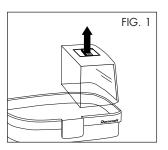
• Remove the Upper Motor Housing from the Reservoir Base, being careful not to let the power cord drop into the base (Fig. 2).
